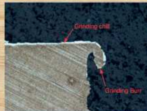
Microphotograph of bandsaw steel showing grinding chill and burr from sharpening.
