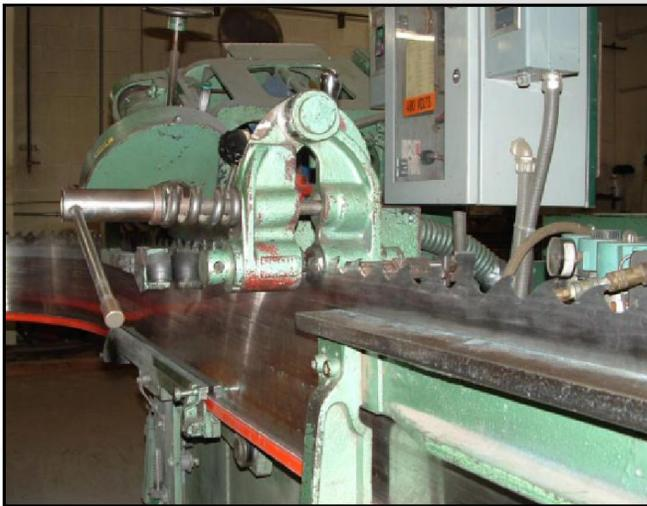
gullet and drawn together under gentle spring pressure. The saw is then fed through the sharpener one more round (not grinding – just feeding) and as each tooth is pulled through the Proctor Roll it gently crimps the bottom of each gullet. This disrupts most of the features that give a crack a place to start, and dramatically reduces cracking.
