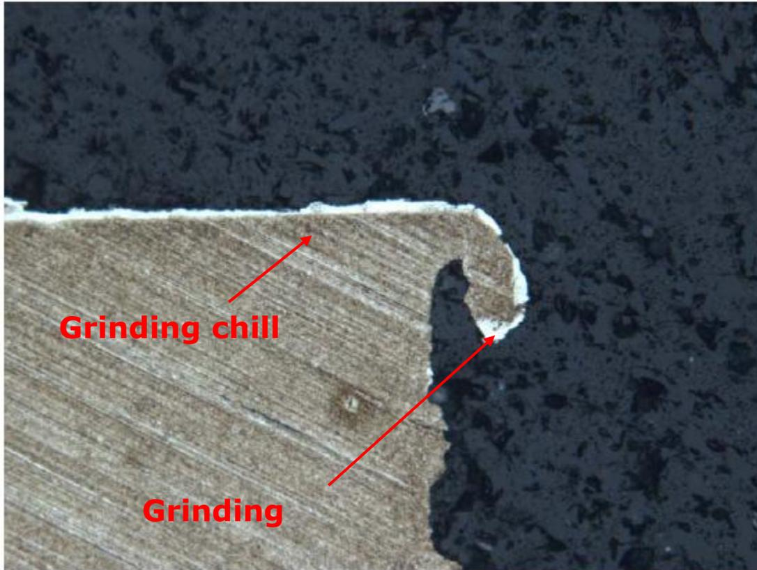
**Figure 1 – Microphotograph of bandsaw steel showing grinding chill and burr from sharpening.**
