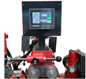
Multi function digital screen presentation of indicator readings and calibration settings.
