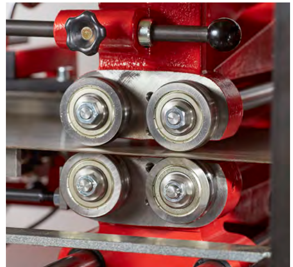
In-line leveling rolls for move steel up or down as based on the indicator readings.
